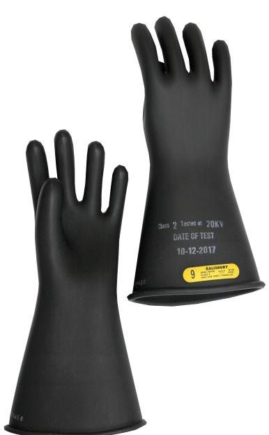
These rubber insulating gloves protect against electrical shock and should be tested every 6 months in accordance with ASTM F496, "Standard Specification for In Service Care of Insulating Gloves and Sleeves" at an authorized safety equipment testing facility. Type I natural rubber. Meet ASTM D120.
